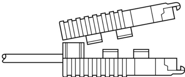
11. Insert one captive screw through a saddle washer and then insert the captive screw with the washer on it, through the hole in the DB25 end of the case. Snap that side of the case closed. Repeat the process for the other side.
