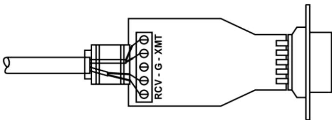
9. Insert the strain-relief assembly, with the wire going through it, into the slot in the bottom half of the modem case and seat it into the recess in the case.
