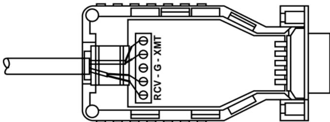
10. Bend the top half of the case to place it over the strain relief assembly. Do not snap the case together.
