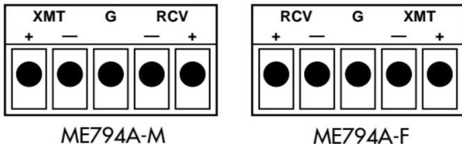
Fig. 3-2. Terminal block configurations for ME794-M & ME794A-F.
