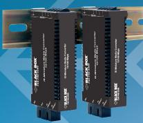
Industiral MultiPower Media Converters. installed on a DIN rail
